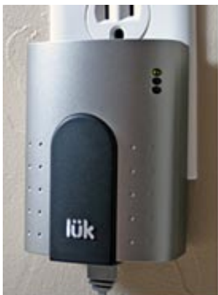
The cord attaches to the Luk Power Source in the wall socket.
