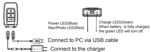
1. Remove the rear covert cap and connect the supplied USB cable into the device.
